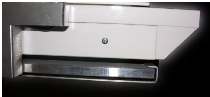
Illustration 6.6: Electromechanical safety switch
